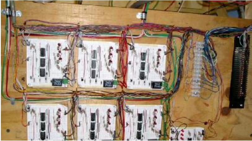
Six of the ten circuit boards for the train detectors and Auto-Stop function.
