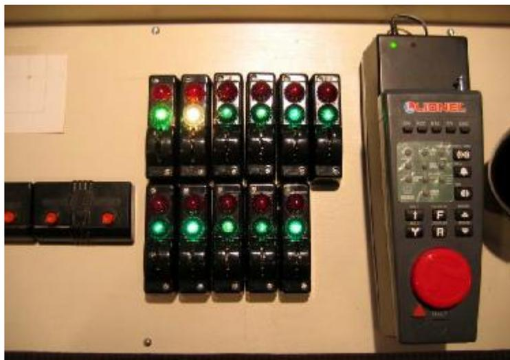
I use *Radio Shack* barrier strips to connect the wiring from the various items (transformers, switch controllers, and uncoupling track controllers) on the control panel to their respective items around the layout.
