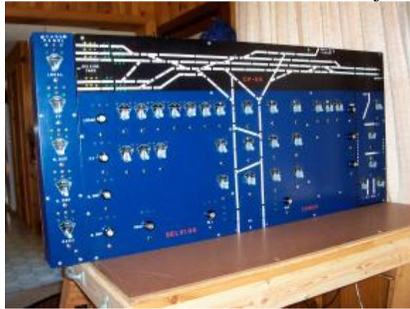
To control the basic flow of traffic, I borrowed, and adapted, a technique from a fellow modeler called "traffic flow request/accept". This set of indicators, levers, and code buttons allows a small panel for the Selkirk Yard Master and a small panel for the Northeast Hudson Dispatcher to communicate to the CP-SK Tower operator on readiness or acceptance of train movements to/from CP-SK. There are corresponding indicators, rotary switches, and code buttons on the CP-SK Tower panel as well.
