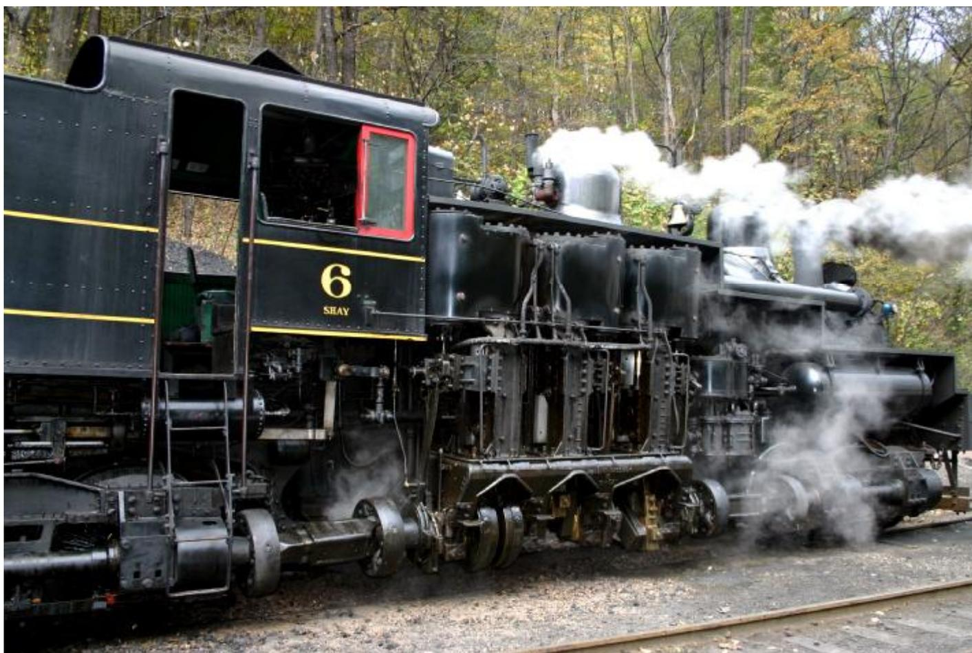
**Shay # 6, a Class C – 150 three - truck shay weighing in at 162 tons and the last Shay ever built, prepares for the morning run up Back Allegheny Mountain to Bald Knob on October 16, 2005. She is the largest surviving Shay locomotive in the world.**
