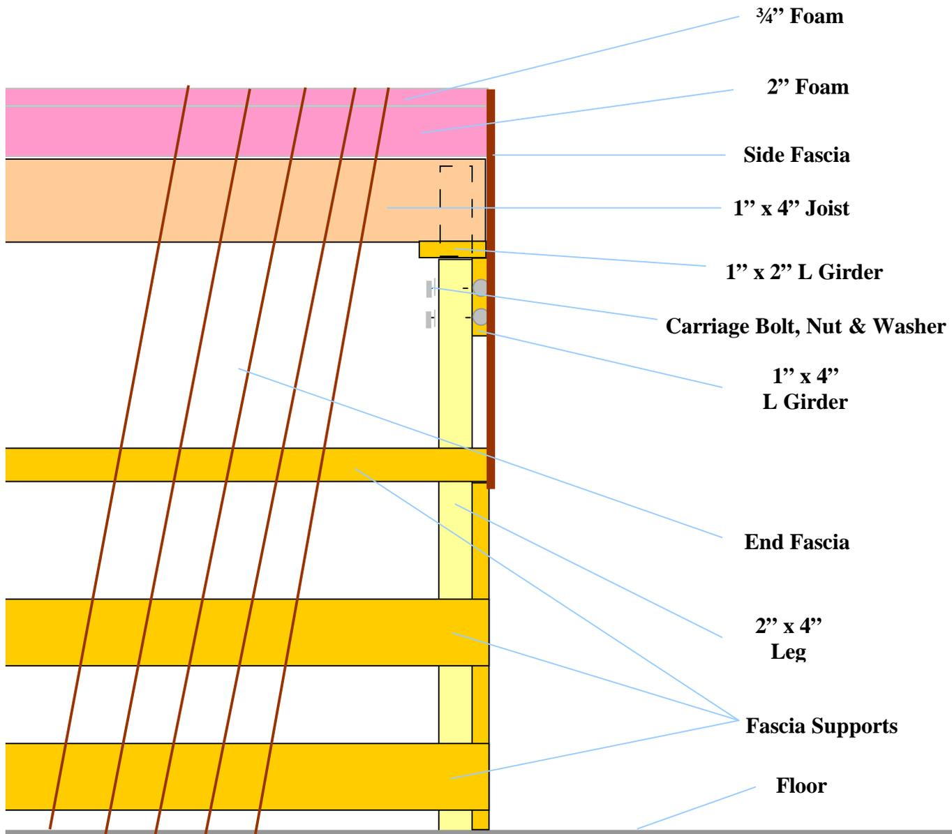
Where a joist is located next to a leg, the joist is attached (screwed) to the leg. The leg is bolted to the 1" x 4" L Girder using carriage bolts, nuts and washers. The fascia on the end will go the floor; where as the fascia on the side will extend about 19 inches from the top allowing access to the cabinets. The legs are bolted to the floor using metal L brackets.
