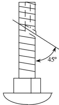
Drilling the holes into the bolts can be tricky business. To make things easier and safer you might want to use a piece of scrap lumber. Drill a couple 1/4" holes and run the bolts through them. Put nuts on them and snug them up. This will hold the bolts so they don't turn and give you something other than the bolt on which to hold.
