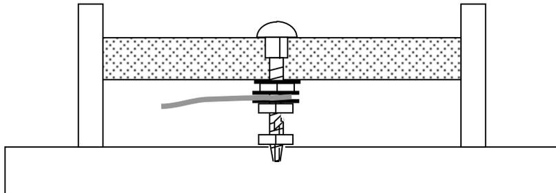
Place a washer than a nut on the bolt and tighten rather tight. Put another washer on the bolt followed by the stripped and looped end of a piece of 12 awg. wire about 12 to 15 inches long. Add still another washer and nut and tighten against the wire. (A scrap piece of "romex" about 24" inches long will fulfill all the wire needs for this project.) Finally, start another nut onto the bolt.
