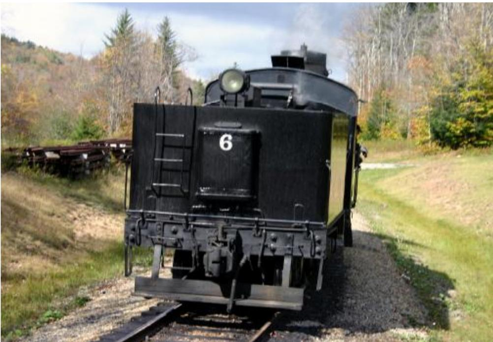
Heisler # 6, a 100-ton Class C – 90, was built for the Bostonia Coal and Clay Products Company of New Bethlehem, PA as their #20. She is a 3-truck Heisler and built by the Sterns Manufacturing Company in 1929.
