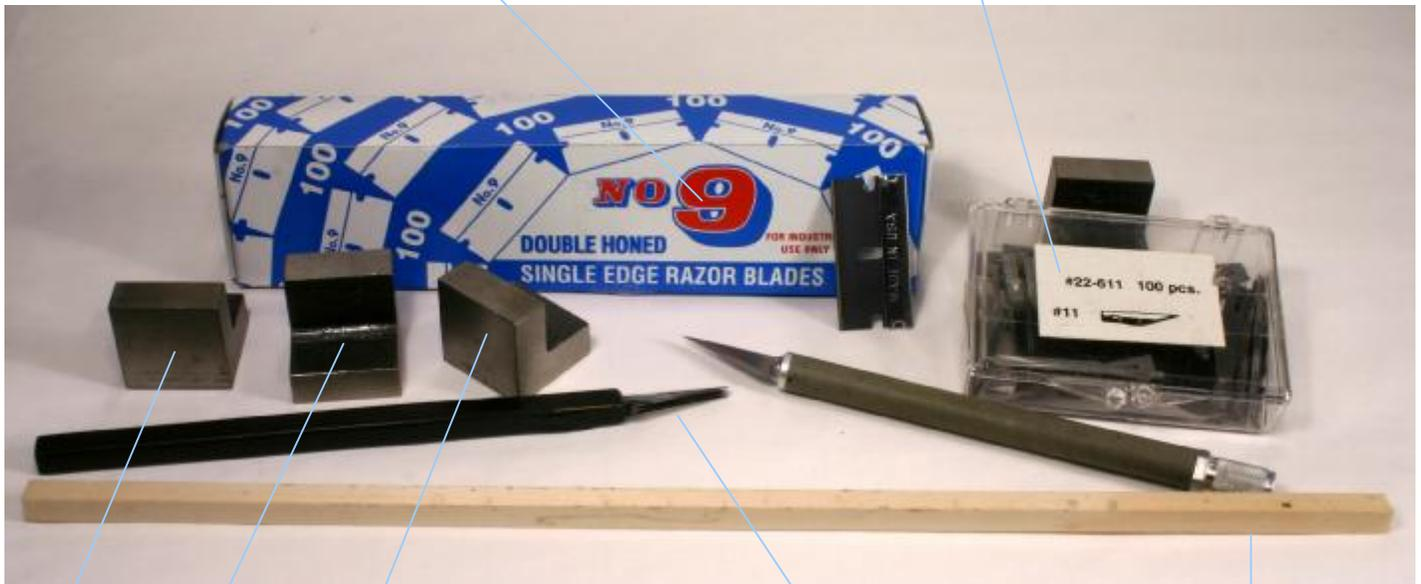
One inch 90 degree angle plates from *Micro-Mark* used to square scale lumber during construction of the sawmill complex structures.
