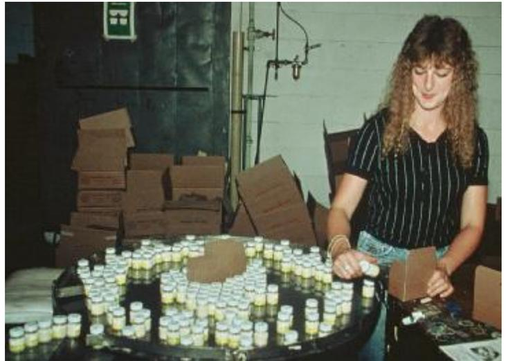
New bottles of *Poly-S Flesh* accumulate on a rotary table for inspection and boxing.
