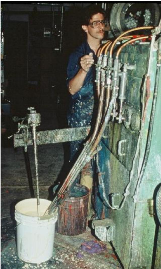
The paint to be bottled is placed in a five-gallon container at the rear of the bottling machine. A stirrer keeps the paint in suspension. Four bottles are filled simultaneously.
