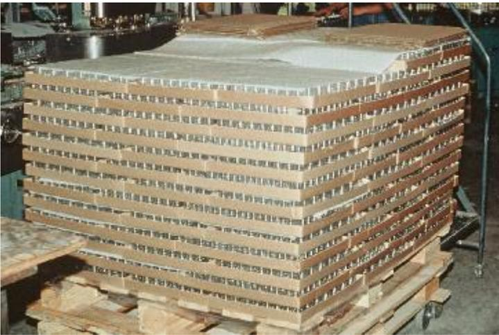
Thousands of one ounce bottles are stacked ready for loading into the bottling machine. The bottles are made of a special glass noted for its clarity.
