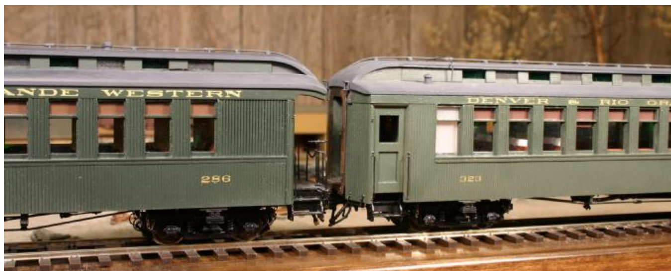
The D&RGW removed the diaphragm on one end of a closed vestibule coach when coupling to an open-ended platform coach as modeled here.
