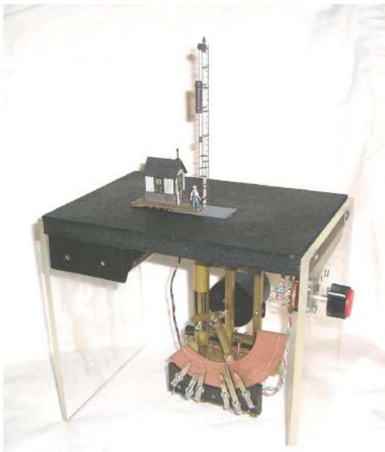
Branch trains have clearance, and three balls – B&M Fitchburg Division trains have clearance. On my layout, the signal is wired through the switch machines so: One ball – routing to the main line, Two balls – routing to the passenger station track, and Three balls – routing to the yard.
