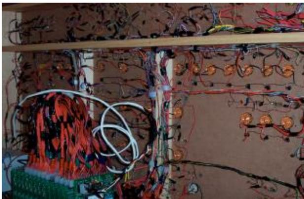
The panel "inputs" into the interlocking mechanism consist of wiring twenty (20) Turnout levers, four (4) diamond-protecting signal levers, ten (10) rotary switches, and thirty-four (34) push buttons, one for each of the previously mentioned items. "Outputs" consist of over 200 LEDs on the Panel Track Diagram for reporting block occupancy as well as turnout, signal, and traffic request lever positions.
